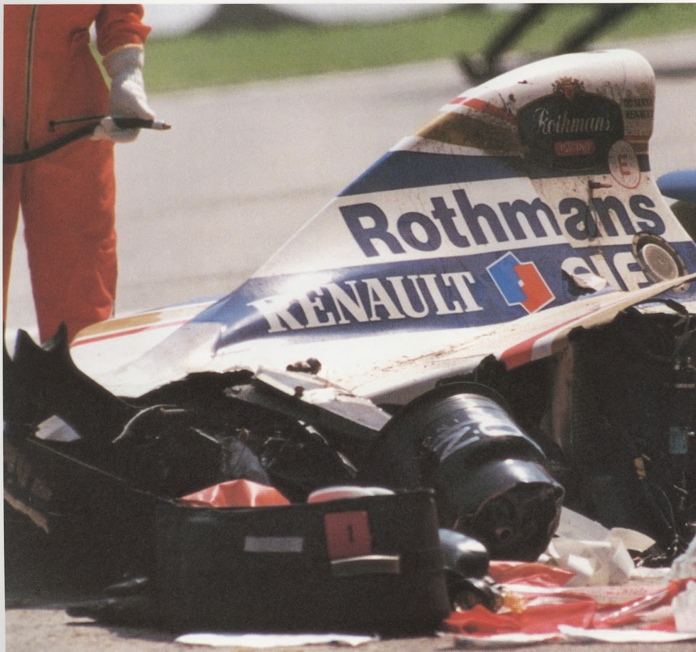
The wrecked Williams FW16: Ayrton Senna died from head injuries caused by suspension parts attached to a wheel which came off on impact.
